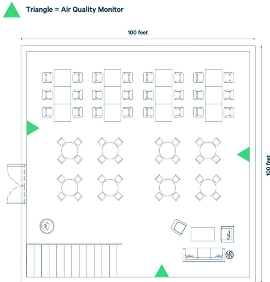
Image 5. A 10,000ft 2 (929m 2 ) open space with three (3) AQMs installed for optimal air data coverage.
