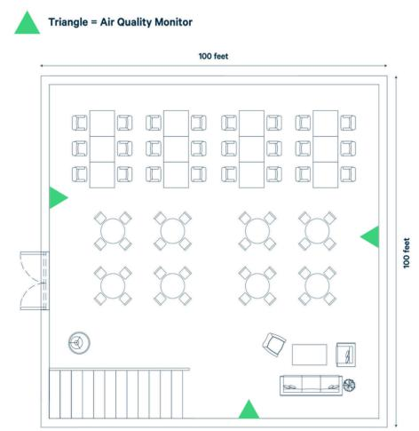
Image 5. A 10,000ft<sup>2</sup> (929m<sup>2</sup>) open space with three (3) AQMs installed for optimal air data coverage.
